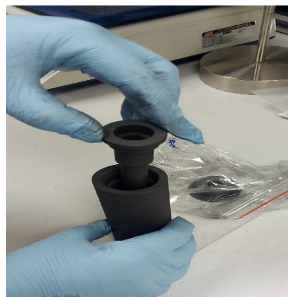
(c) Putting the thermometer well inside the crucible after the first filling of the mixture
