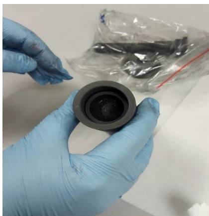
(b) Filling the crucible with the Fe-C mixture
