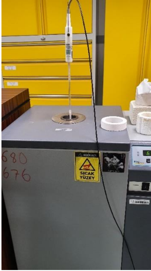
Figure 2. a) Calibration of the HTSPRT in Al Fixed point. b) Connection with thermometric bridge and measurements taken from software.
