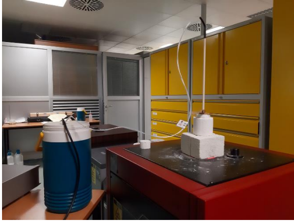
Figure 3 Constructed thermocouple – measurement on Ag fixed point
