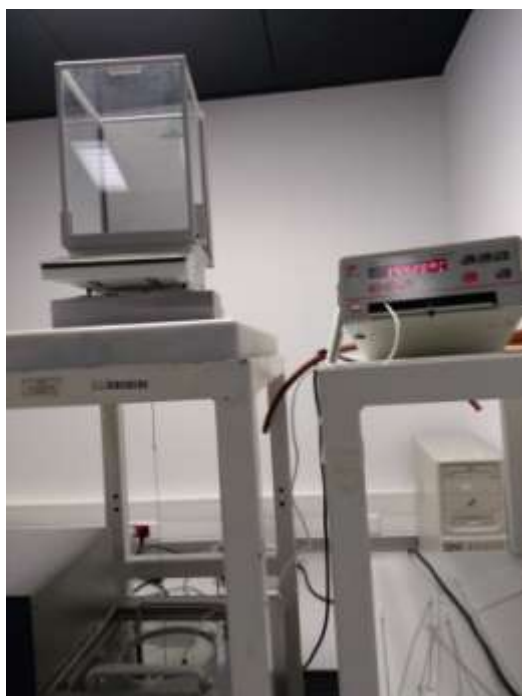
Fig.1. Manual Solid Density measurement system at UME
