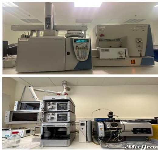
Figure 1. Preparation of stock solutions; Figure 2. GC-MS/MS (up) and HPLC-MS system (down);
