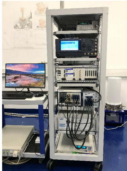
Fig.3.1 the Cryocooled PJVS system
