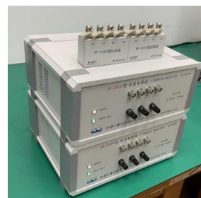
Fig. 6.1 The new type active simulated inductance standards proposed by NIM
