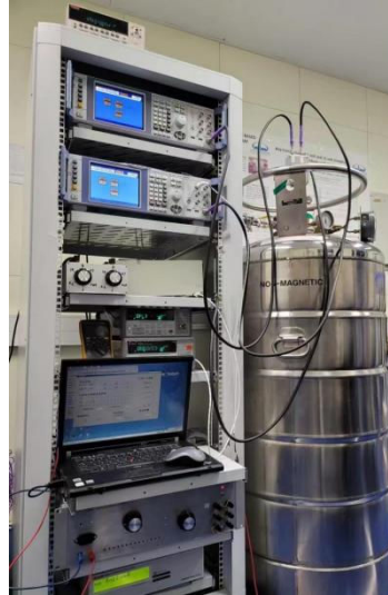
Fig. 3.2 The improved low-voltage Josephson standard developed at NIM based on the differential frequency Josephson array
