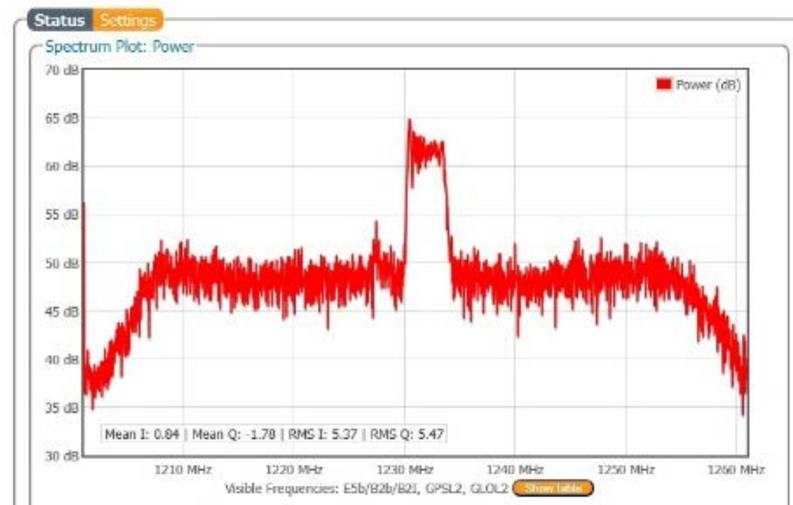
PolaRx5TR Spectrum power with anomalies
