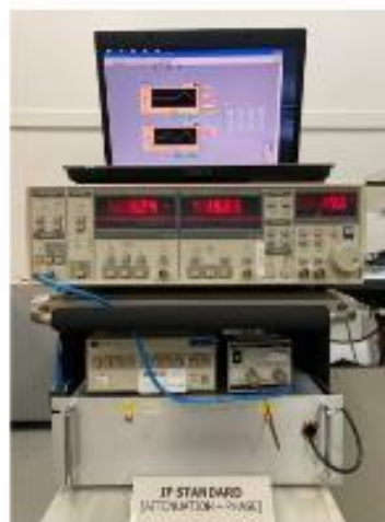
Fig. 8-2 Block diagram of the primary standard system for RF/MW attenuation and phase-shift (left) and picture of its working standard system. (right).
