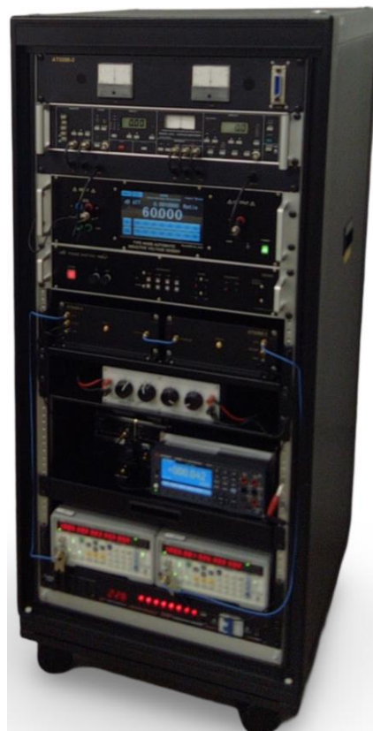
Fig. 8-1 Photograph of the commercialized NMIJ RF/MW attenuation measurement system.
