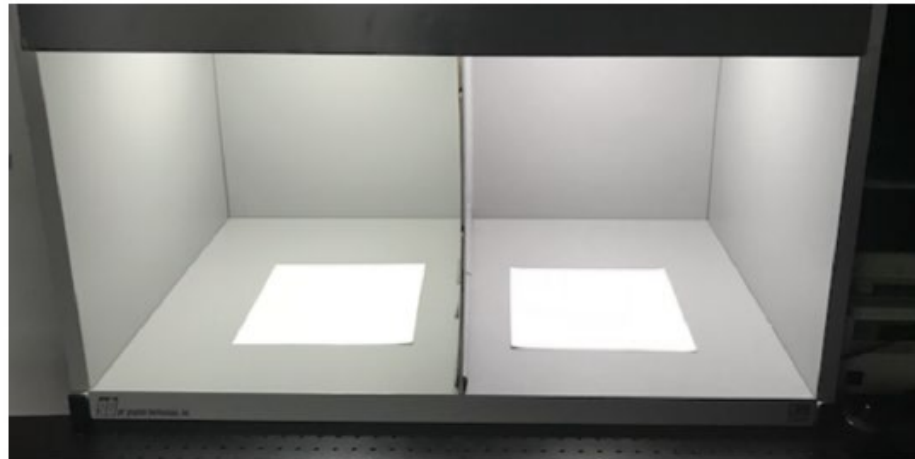
Figure 6 – Spectrally-Tuneable Double Booth used for the experiment
