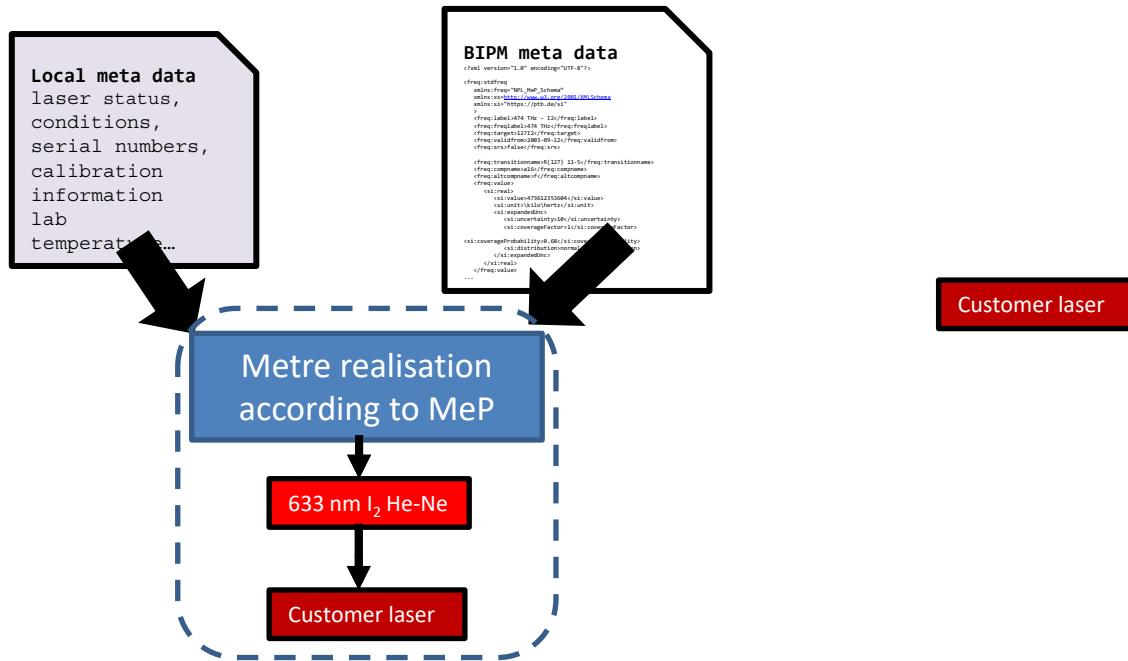
Laser is returned to customer, NMI makes the calibration data (including meta data) available from its server (or supplied on digital certificate)
