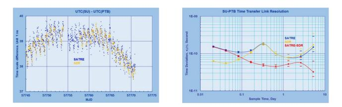
noise component for SDR. Diurnal component still presents both in SATRE and SDR data. Red curve at the right figure demonstrates random residuals in SATRE-SDR links. If one will succeed in suppression diurnal component SDR link performance will be considerably better than  $1 \times 10^{-10}$  s for any sample time starting from session repetition up to a few days.
