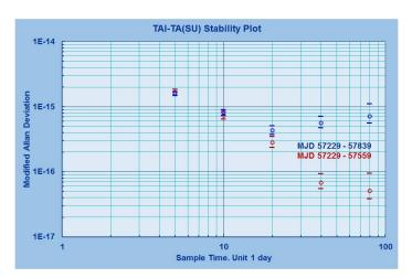
fountain standard reliable and correct operation up to July 2016 we got very impressive figures of TA(SU) time stability relative to TAI. For the whole period of estimations 2015 up to beginning 2017 TA(SU) stability level looks much more moderate, first of all due to bad CSF02(SU) operation.
