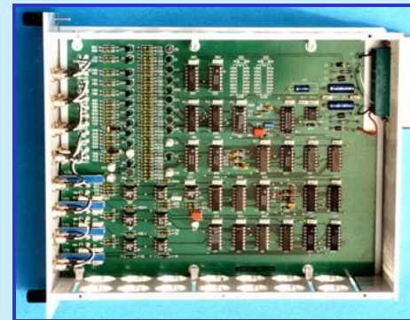
Inner view of the coincidence unit
