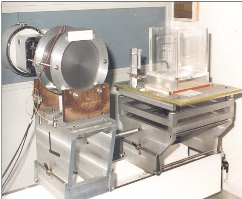
BIPM ionometric standard of absorbed dose to graphite
