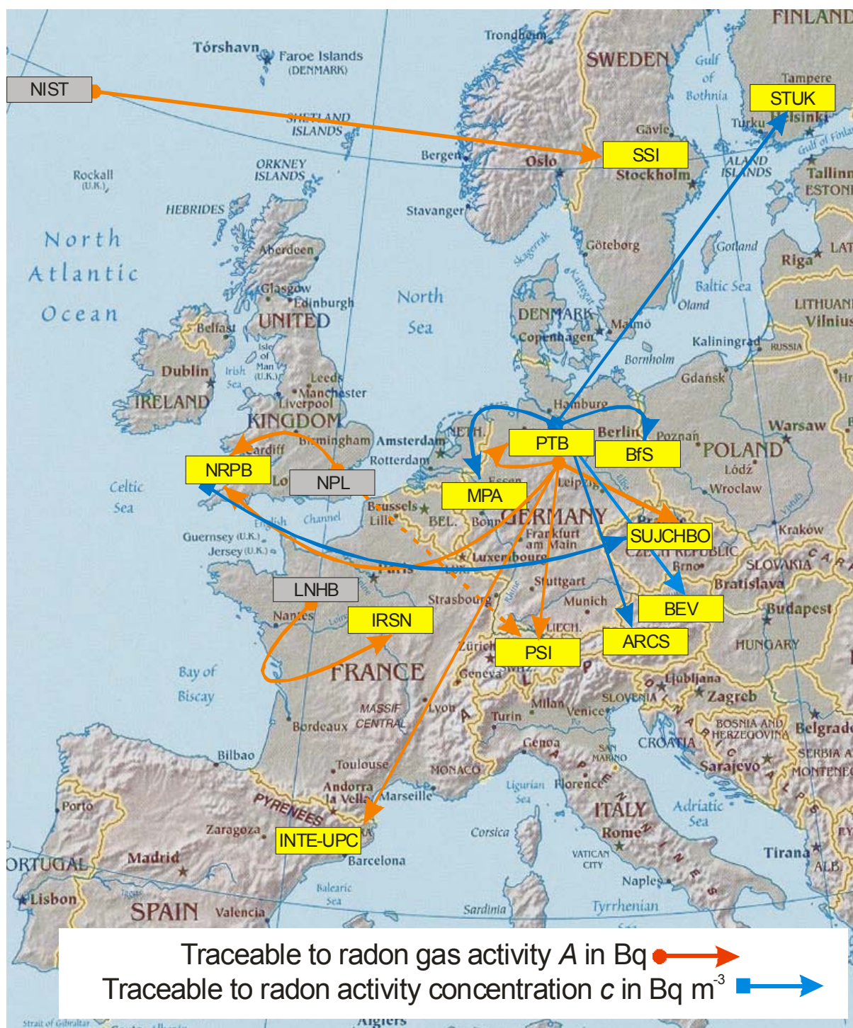
Figure 2: Traceability chains for the radon activity and the radon activity concentration of the participants. The arrows show the established transfer of the quantity, by sending from the institute at the starting point either a gas standard or a reference instrument to the institute at the ending point. Exception is SSI using a Ra-226 standard solution traceable to NIST as activity standard.
