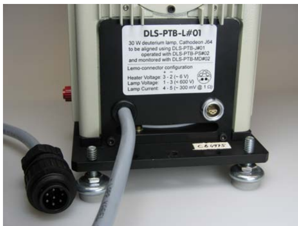
Figure A.6 Connector at the lamps back to measure the electrical parameters of the lamp
