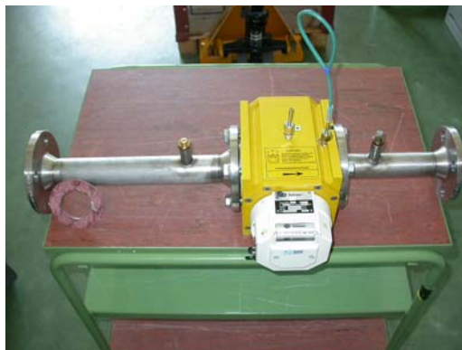
Fig. 2.1: Picture of the used transfer standard with the down and upstream pipes.
