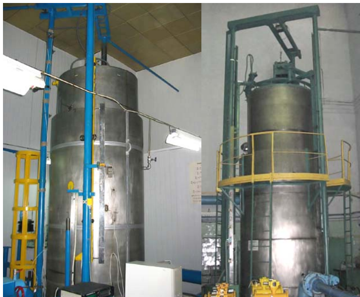
Figure 11: Provers appearance State gas flow standard DETU 03-01-96 – left, gas flow standard RKDU-0,44 – right
